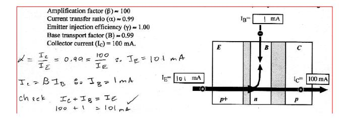
(4) Draw a common emitter PNP BJT circuit (see image at right for an example), and for Vbe have a 10 k $\Omega$  resistor, and for Vce have a 500  $\Omega$  output resistance. Assume the amplification factor is 100. If we apply 1 V to forward bias the emitter base, and 20 V across the emitter and collector to setup the base-collector as reverse biased, what will the voltage drop be:
